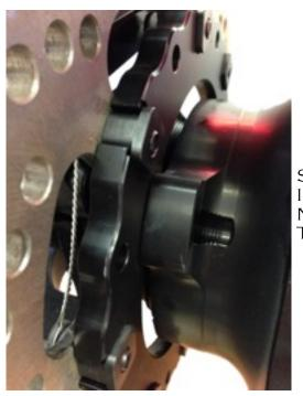
STEP 2 INSTALL THE ROTOR AND THE T-NUTS AS SHOWN. JUST FINGER TIGHTEN THE BOLTS FOR NOW.
