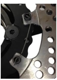
IF AT FIRST THE ROTOR SEEMS A LITTLE TIGHT IT IS BECAUSE THE T-NUTS HAVENT HAD ANY FORCE ON THEM FROM THE BRAKES TO "ALIGN" THEM WITH THE SLOTS. ALWAYS CHECK EVERYTHING TO MAKE SURE IT IS TIGHT AFTER A FEW SLOW LAPS OF BEDDING THE BRAKES IN. NEVER RUN AT HIGH SPEEDS WITHOUT RE CHECKING ALL THE BOLTS ON YOUR BRAKING SYSTEM INCLUDING BRACKETS, ADAPTERS, CALIPERS, LINES AND ANYTHING ELSE RELATED.
